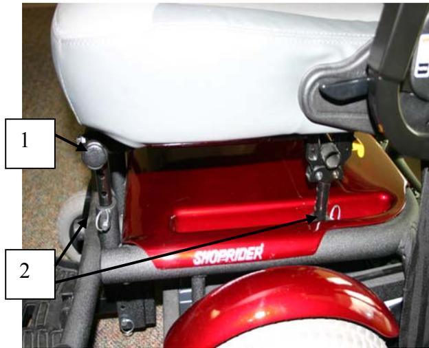
2. Adjustment pins that can be used to adjust the height of the seat to fit the user.
